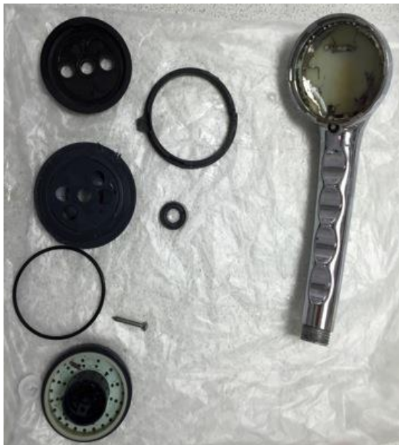
Dismantled adjustable showerhead with areas of low flow and EPDM rubber components. There was a distinct smell of stagnation when disassembled
